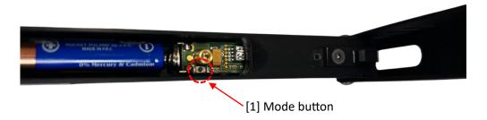
3) Use the allen key you used for loosening the barrel cover. Place it on the top of the button and load the gun. Now gently press it (Do not push too hard or you will break the button. You will hear and feel a little click.) Now hold the button and pull the trigger. The gun should emit laser and change its mode
